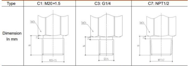
Note: Common threads are M20×1.5, G1/4, G1/2, M14×1.5, NPT1/4 and NPT1/2. Special threads can be customized for batch order.
